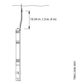
Fig. 4 Vertical installation
