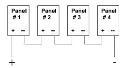
Fig. 21 Solar panel wiring in series
