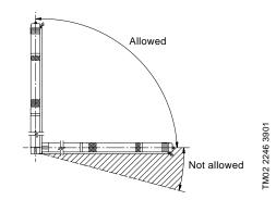
Fig. 6 Installation of SQF pumps
