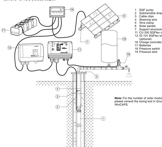
Fig. 14 SQFlex Solar with back-up batteries
