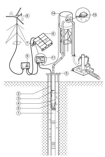
Fig. 19 SQFlex Combi with CU 200 and level switch
