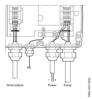
Fig. 32 Electrical connections
