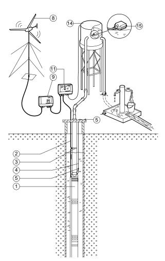
Fig. 17 SQFlex Wind with CU 200 and level switch
