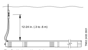
Fig. 5 Horizontal installation
