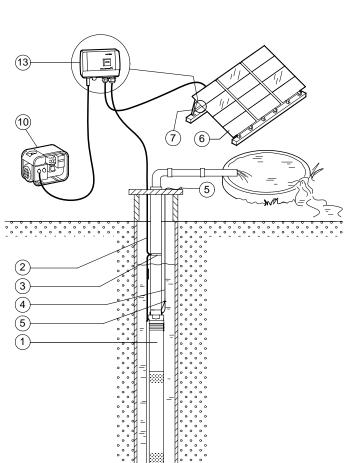
Fig. 13 SQFlex Solar with back-up generator
