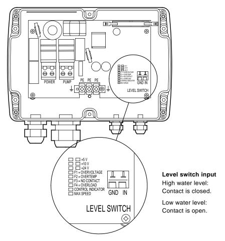
Fig. 26 Electrical connections, CU 200
