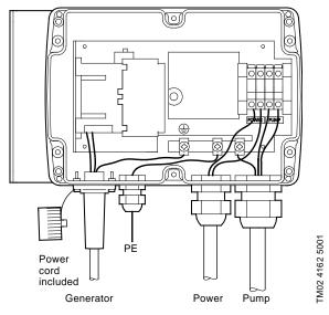
Fig. 30 Electrical connections
