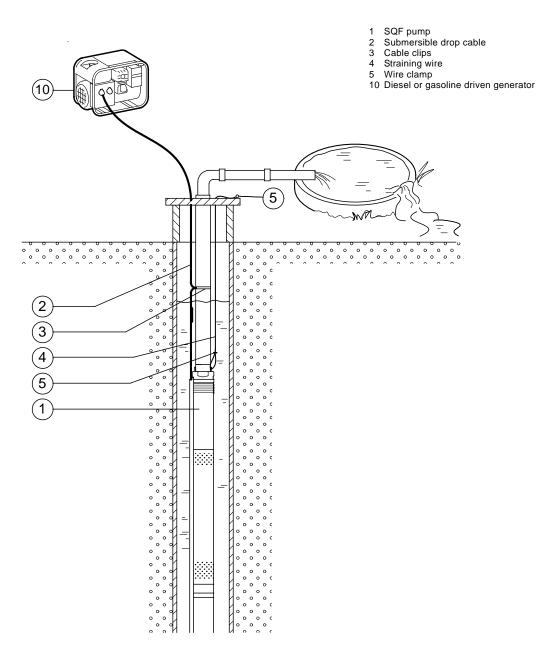
Fig. 20 SQFlex system with generator as power supply.
