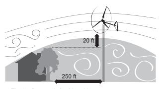
Fig. 16 Proper wind turbine siting
