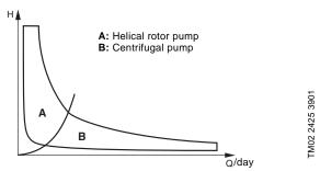
Fig. 1 Performance ranges for helical rotor and centrifugal pumps
