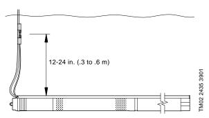
Fig. 7 Horizontal installation
