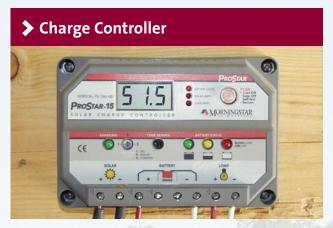
Morning Star PS15M-48V Charge Controller includes connections for solar input, battery output, and load output to the CU 200 and SQFlex
