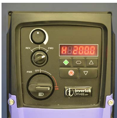
Fig. 9d Switch 3 set to 200 Hz
