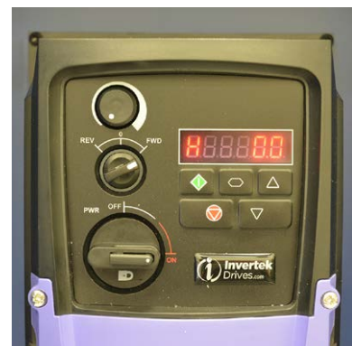
Fig. 9c Switch 2 set to FWD
