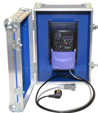
Fig. 8 Vertical installation of the converter
