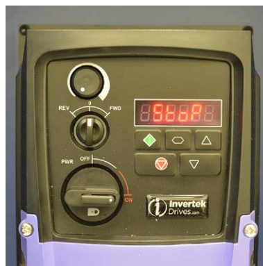
Fig. 9b Switch 1 set to ON
